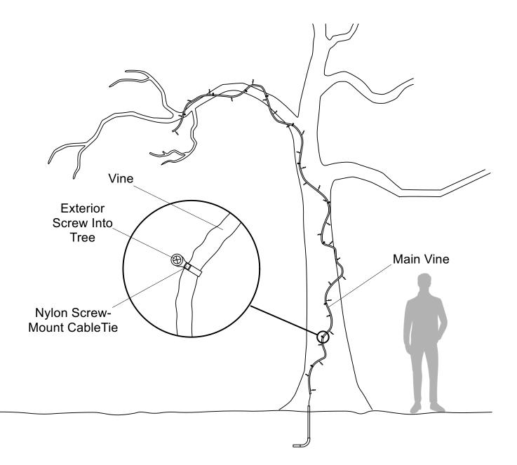
**Step 3:** Once the Main Vine is installed, you can start attaching branches. To create a branch, cut off a segment of vine (3'-5' long is typical) using wire cutters. Always cut at the insulated trunk, not at one of the tentacles. Next, attach the branching vine to the Main Vine with cable ties, then twist a tentacle from each together to create the electrical connection. Touch up the cable ties with paint as needed to blend.
