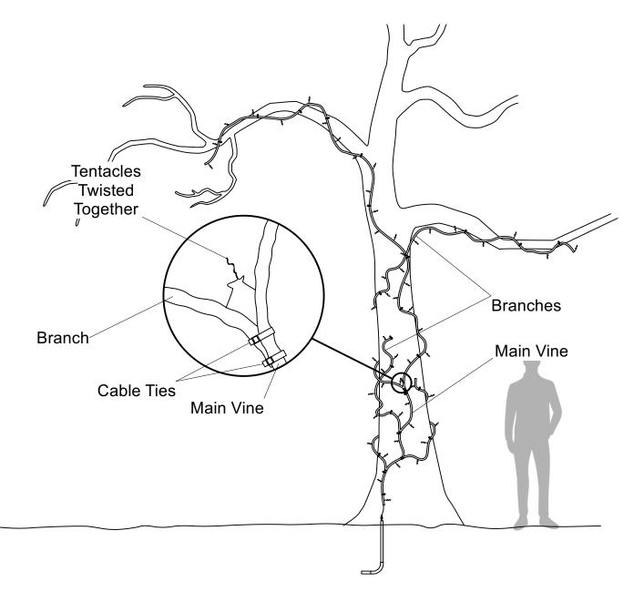
**Step 4:** Finally, follow the instructions included with your electric fence charger to correctly install and ground the unit. Run the positive feed in conduit to the Main Vine and attach it to the Hookup Wire at the end of the vine using a wire nut.
