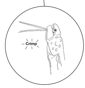
**3. Crimp:** After you have snipped the wires you wish to connect, scratch away 1 inch of paint and **CRIMP** the ends together using the duplex ferrules provided. Crimp the ferrules just enough so they will stay on the wires using a large pair of pliers.
