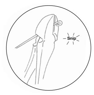
**2. Snip:** Next, using your rebar as a yardstick, space the grass clumps 30" (for Econo/Short Grass) or 36" (for Tall Grass) apart base-to-base. You will attach the first clump to the power supply, then link them clump-to-clump above ground by snipping and crimping: Using wire cutters, **SNIP** off the looped end of the grass wire(s) that you wish to link with the next clump(s).
